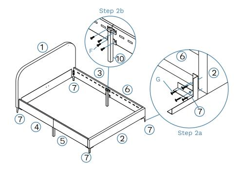
2a: Attach 4 x legs (7) to assembled frame and secure with 16 x bolts (G). Tighten with a screwdriver.
