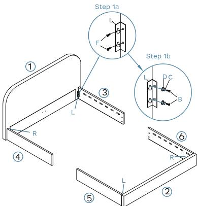
1a: Attach 1x left plate (L) and 1x right plate (R) to panels [1], [3] and [4] and secure with 4x spring washers (D), 4x washers (C), 4x 25mm bolts (B), 4 x20 bolts (F). Tighten with Allen Key (T2) and (T3). Do not completely tighten the screws until the complete frame is built.
